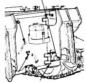
HULL REAR DOOR HINGES, HOLD-OPEN LATCH, HANDLE. AND HOLD-OPEN ROD HINGE AND PIN
