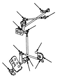
ACCELERATOR PEDAL AND HAND THROTTLE CONTROL LEVER
