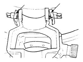
M145 TELESCOPE MOUNT CLAMPING CATCHES
