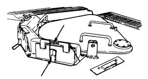
M45 DRIVER'S PERISCOPE COVER PINS, LATCHES, AND HINGES
