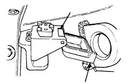
M140 ALINEMENT DEVICE MOUNT, COVER, DOVETAIL DOOR WEDGE, AND CLAMPING CATCH
