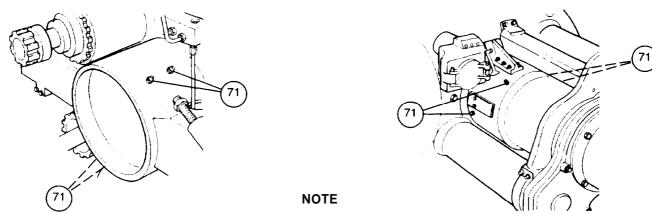
For clarity, inside of mount is shown out of howitzer. Right side lubrication fittings are shown on top and left side lubrication fittings are on bottom.
