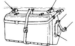
LEFT AND RIGHT CANNONEER'S SEAT ASSEMBLIES HINGES AND PINS (M109A4/M109A5)
